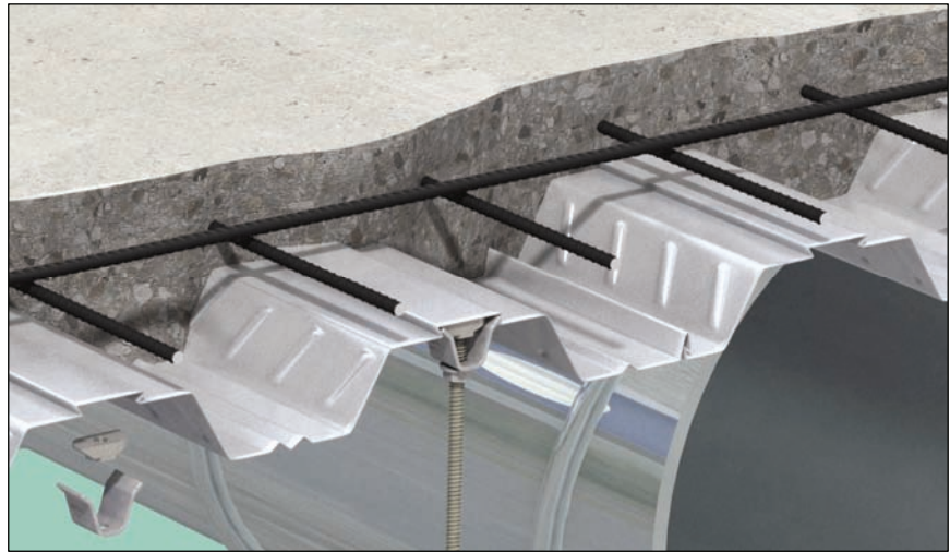
Figure 15: A cross-section of a composite concrete deck.
