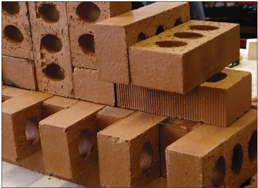
Figure 21: Perforated blocks with dense structure.
