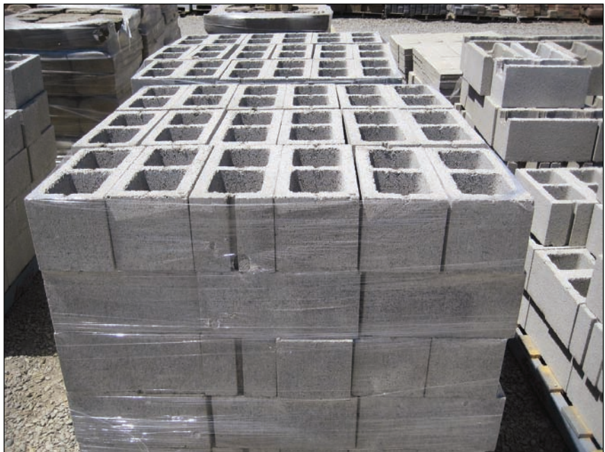
Figure 22: Perforated blocks with porous structure.
