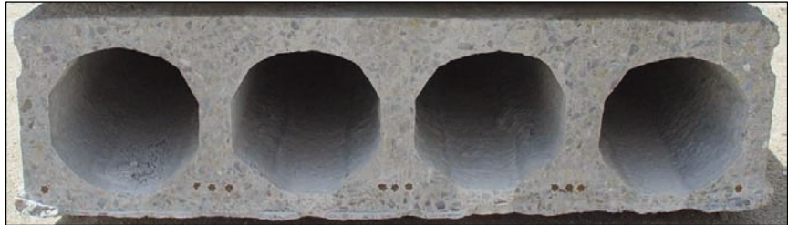
Figure 13: A cross-section of a hollowcore concrete slab showing four voids and three sets of post-tensioning tendons.
